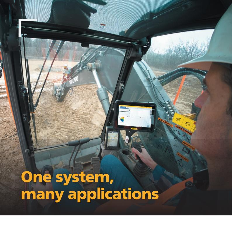
The **Trimble** Siteworks Machine **Guidance Module** is a versatile, low cost solution for machine guidance and layout that enables contractors to use the same hardware and software to perform a variety of tasks on the job site both on and off machines.
